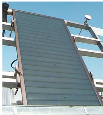
Figure 1: Picture of the collector thermo|solar 300N2P mounted on the efficiency test facility (Tracker) of Fraunhofer ISE
