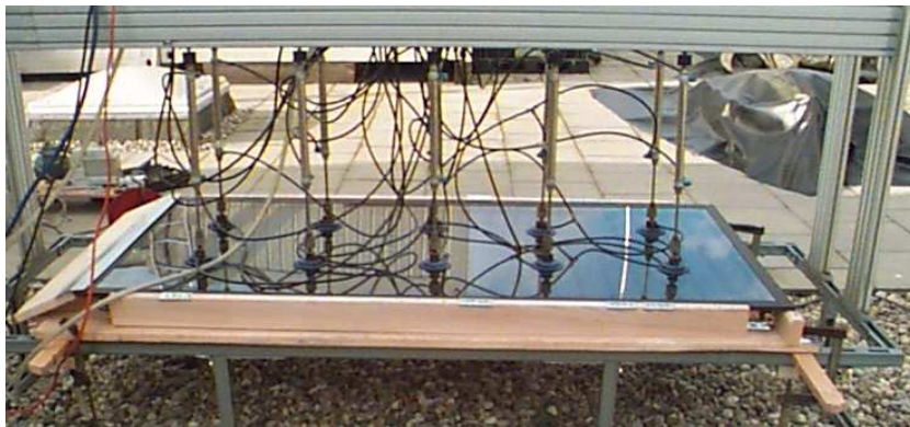
Figure 9: Position of additional fixings for regions with high wind speed
