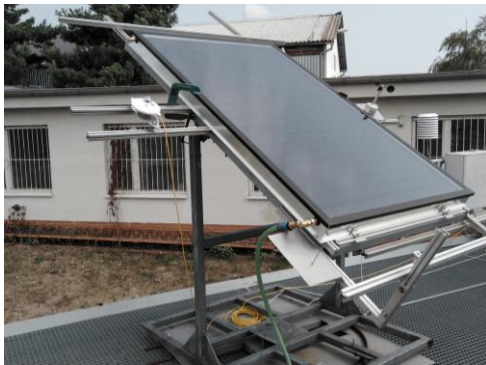
Exposure test and Internal thermal shock
