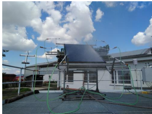
Exposure test and external thermal shock
