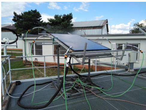
Rain penetration test
