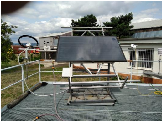
Exposure test and Internal thermal shock
