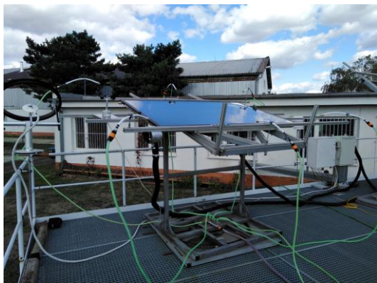
Rain penetration test
